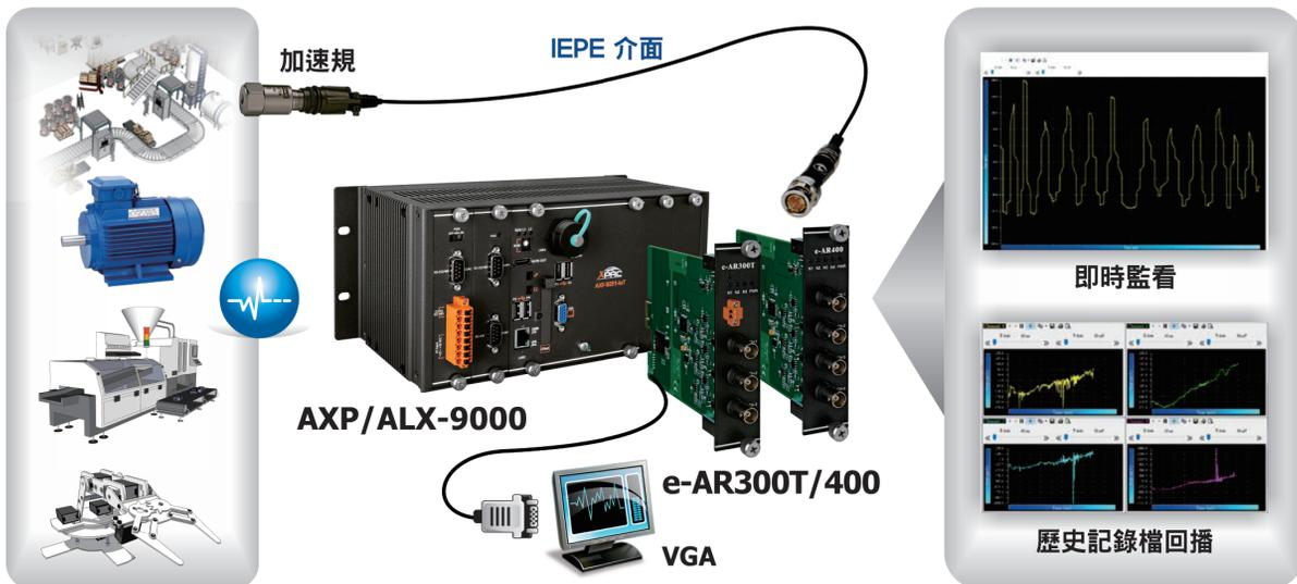
e-AR300T / e-AR400 is a high-performance dynamic signal data acquisition module developed for mechanical vibration measurement. Each channel provides 200 KHz simultaneous sampling. The product has a built-in 3 mA excitation current for integrated electronic density (IEPE) power supply and 16-bit analog-to-digital conversion, and all collected signals are sent to the SD card for user card analysis. It is the best choice for vibration measurement applications.
