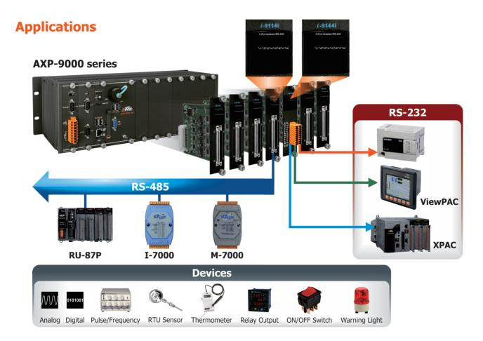
To get more RS-232/485/422 ports, user can plug one or more "multi serial port module" in the I/O slot.
