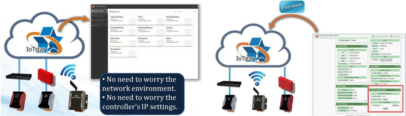
Collect the Historical and Real-Time sensor data (and Power data) from the WISE/PMC/PMD controllers, and import them into the Database. User can modify the database data to change the status of the DO/AO channel of the sensor connected to WISE/PMC/PMD through the SQL command. Please note: IoTstar currently support MS SQL.
