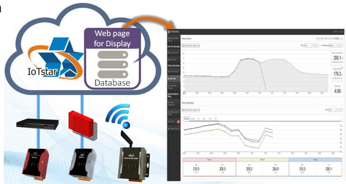
The users can quickly setup the Data pool for their IoT system by receiving and importing the sensor data into the Database through the IoTstar. User can analyze the sensor data with analysis tool, the status can be known, and the necessary actions can be taken in advance to avoid possible damage.
