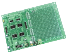
面包板 Board X002 (114mm x 170mm)
